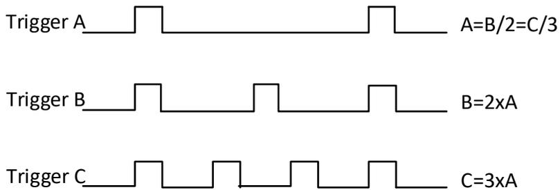
Inserting one (2-1) pulse between every two pulses of trigger A becomes trigger B; inserting two (3-1) pulses between every two pulses of trigger A evenly creates trigger C. Frequency-wise, they result in  $B=2xA$  and  $C=3xA$ . This is how the multiplier works.
