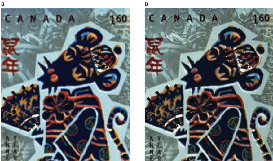
Figure 5. A stamp captured by Piranha Color trilinear camera (a) versus Spyder3 Color bilinear camera (b).
