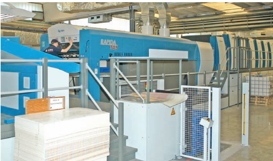
Figure 8. The Rapida 145 press by Koenig & Bauer AG of Würzburg, Germany, uses the Piranha Color 4k camera in its QualTronic ColorControl unit to measure and control color density in-line.
