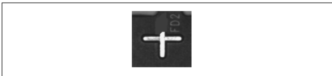
Figure 82. Fiducial with Missing
