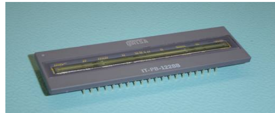
Figure 1. Photograph of the IT-PB-12288 12K 5 \mu\text{m} 320 MHz CCD.
